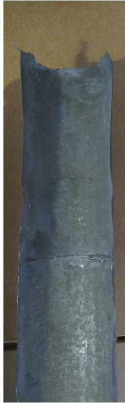
12a-b: traces of sand-casting
